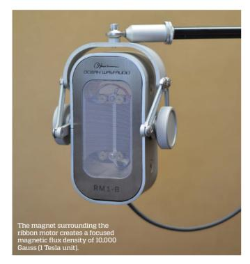
cean Way Audio's RM1-B is the company's latest iteration of Cliff Henricksen's RM1 active, bi-directional ribbon microphone. The RM1-B has the RM1's motor assembly with a 1.77-micron-thick aluminum ribbon. It uses a discrete phantom-powered preamplifier designed to Henricksen's specifications.
